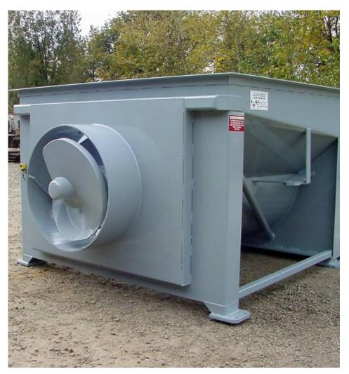
You can google "Auger Compactors" for more information; there are now a number of manufacturers producing auger compactor equipment. The key advantage of the auger compactor equipment is that feed can involve a larger number of waste types than can go into a ram compactor. Also, there is no cycle time; auger compactor-feed is continuous. For more information, call Komar Auger System, Del Miller at 717-880-1109.
